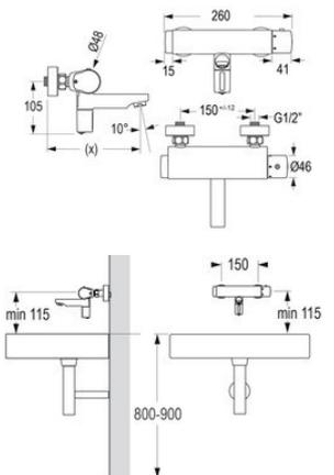
Touchless, electronically controlled wall-mounted faucet for surface installation:
